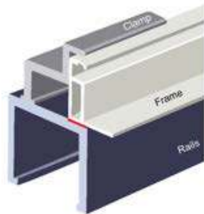
The frame overlap the rails the overlapping distance must \geq 20 mm.
