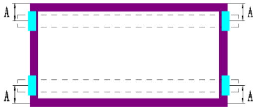
Use 4 clamps on the short side. Mounting rails run parallel to the long side frame.
